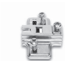
Asymmetric mounting plate for central panel. Fixing by dowels and selftapping screws. Vertical adjustment.
